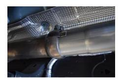
2. Remove clamp from factory head pipe using a small flathead screwdriver to bend up the retaining clip and then install onto new head pipe (Item A).
